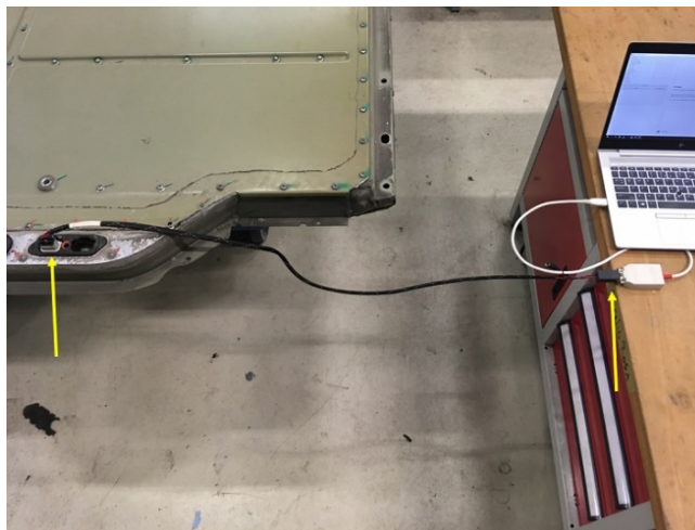
Figure 4 - Connection to PCAN-USB adapter (Model S and Model X)
